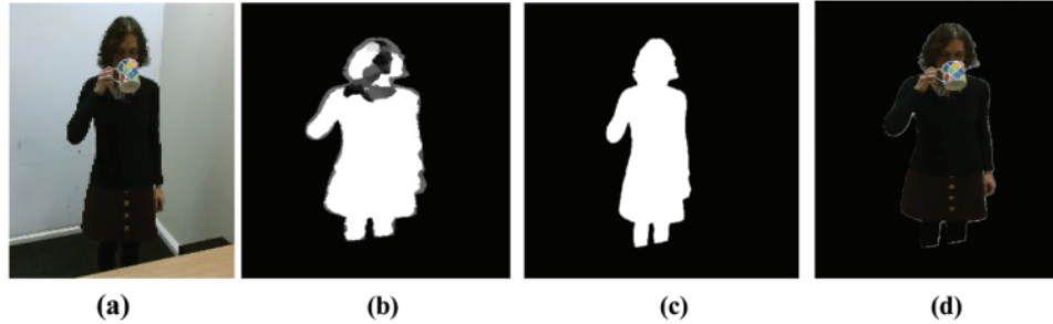
Figure 2: Human silhouette detection of RGB images: (a) Original image, (b) Subtracted frame, (c) Binary silhouette, and (d) Resultant RGB silhouette
