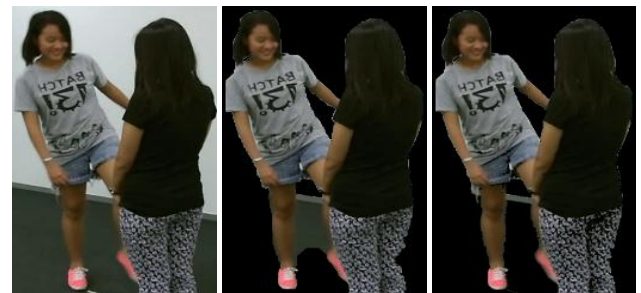
Figure 2. Segmentation results on RGB images showing (a) the original RGB image, (b) GrabCut output, and (c) segmented humans after applying floor mask.
