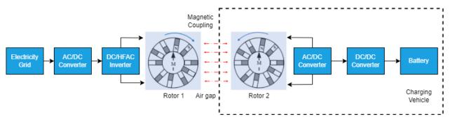
Figure 8. Architecture of an MGWPT system.
