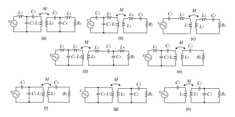
**Figure 16.** Hybrid and advanced compensation networks [50]: (a) LCC/LCC, (b) CCL/LC, (c) LCL/LC, (d) LCL/LCCL, (e) LCC/S, (f) SP/S, (g) P/PS, and (h) S/SP.
