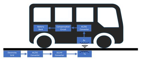
**Figure 1.** General structure of a static wireless charging system for EVs. The coils may be replaced by capacitive pads in capacitive coupling.
