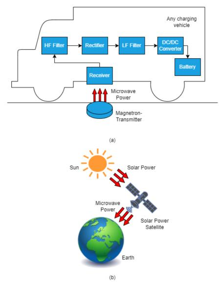
**Figure 10.** WPT by microwave charging. (a) A microwave charging system for EVs. (b) Microwave power transmission using solar power satellites has been proposed by researchers from JAXA.
