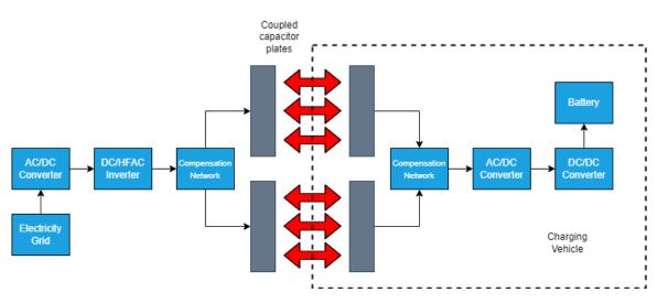
Figure 5. Structure of a CPT system.
