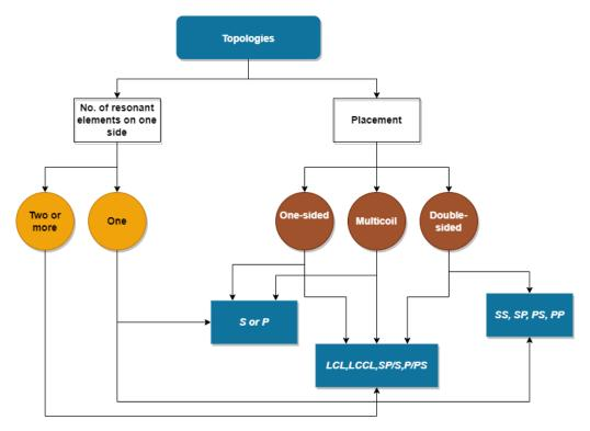
**Figure 15.** Classification of compensation topologies based on the number of resonant elements in either the transmitter or receiver and the location in the system.
