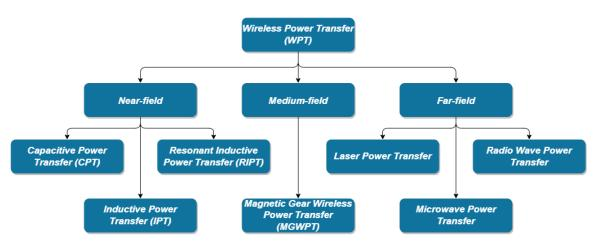
Figure 3. All wireless power transfer methods mentioned in the literature relevant to wireless EV charging.
