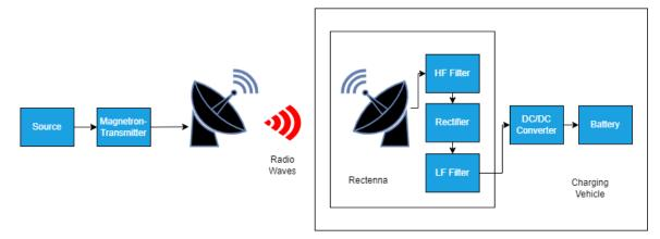
Figure 11. A radio wave charging system.
