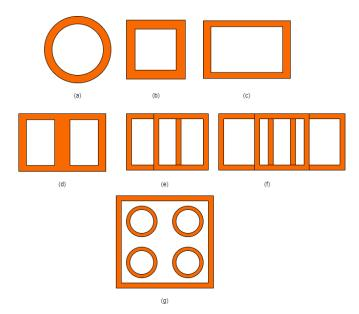
**Figure 13.** Various coil shapes that are typically used: (**a**) circular, (**b**) square, (**c**) rectangular, (**d**) DD, (**e**) BP, (**f**) DDQ, and (**g**) QDQ.
