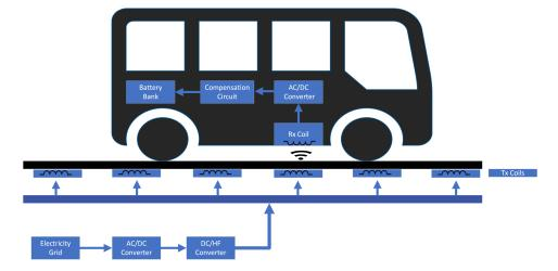
Figure 2. General implementation of a dynamic wireless charging system for EVs.
