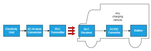
Figure 9. A laser charging system.
