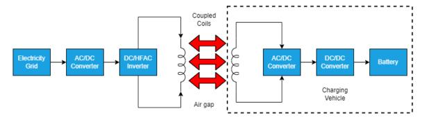
**Figure 6.** Structure of an IPT system. Compensation networks can be added before the primary and after secondary windings.
