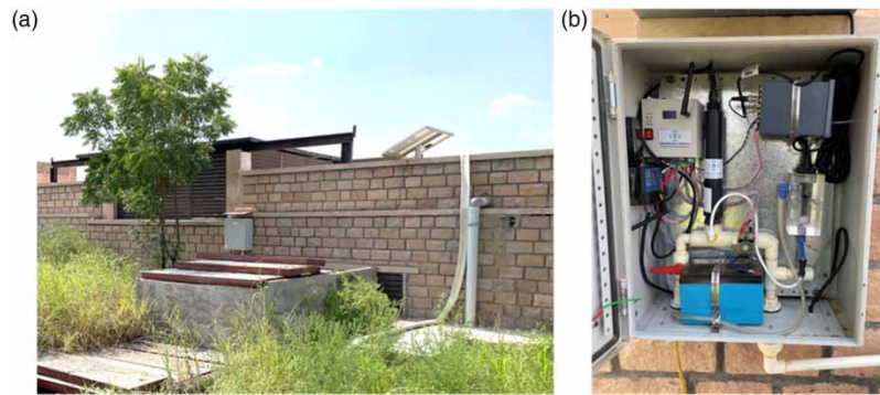
Figure 6 | Quality node and its components. (a) Above the ground unit with solar panel. (b) IP67 enclosure for housing IoT devices and other components.
