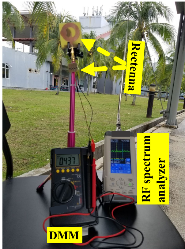
Figure 6. The ambient measurement setups of the proposed RF rectifier prototype.
